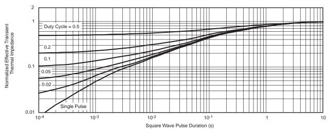
Normalized Thermal Transient Impedance, Junction-to-Foot
