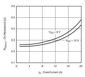
On-Resistance vs. Drain Current and Gate Voltage
