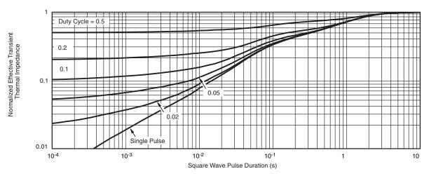
Normalized Thermal Transient Impedance, Junction-to-Foot
