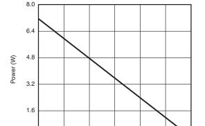
$T_C$  - Case Temperature (°C) **Power, Junction-to-Foot**
