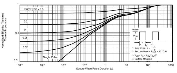
Normalized Thermal Transient Impedance, Junction-to-Ambient
