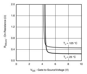
On-Resistance vs. Gate-to-Source Voltage
