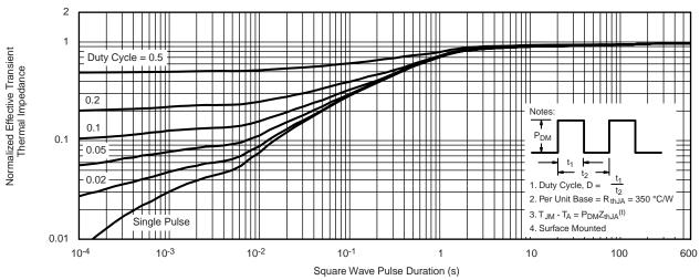
Normalized Thermal Transient Impedance, Junction-to-Ambient
