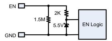
Figure 2. Zener Diode between EN and GND
