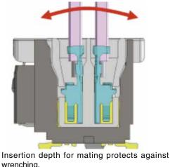
wrenching. Thick and robust outer wall provides higher strength and prevents cracking.
