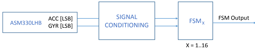
Figure 2. State machine in the ASM330LHB
