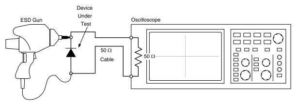
Figure 8. Diagram of ESD Clamping Voltage Test Setup
