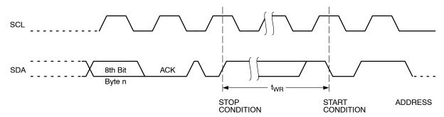
Figure 7. Write Cycle Timing
