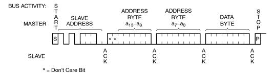
Figure 6. Byte Write Sequence
