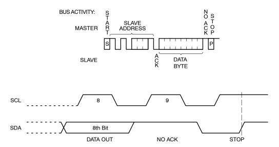
Figure 10. Immediate Read Sequence and Timing
