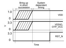
Figure 16: Sequencing of power supplies and RST\_N
