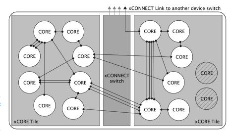
Figure 6: Switch, links and channel ends
