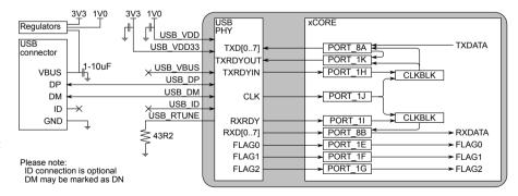
Figure 11: Bus powered USB-device
