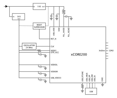
Figure 2: Simplified Reference Schematic
