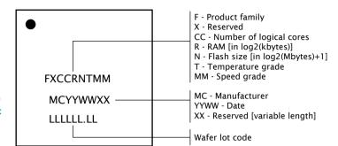
Figure 30: Part marking scheme
