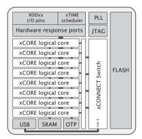
Figure 1: XUF208-256-TQ64 block diagram
