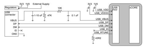
Figure 12: Self powered USB-device
