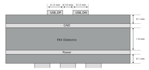
Figure 18: Example USB board stack
