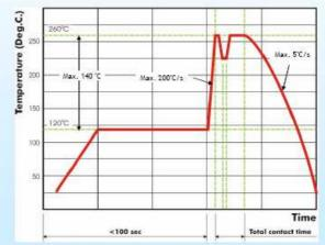
Fig. 2 Recommended wave soldering profile for SMT process with SnAqCu series solder.
