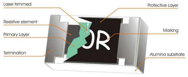
Fig 1. Construction of Chip-R
