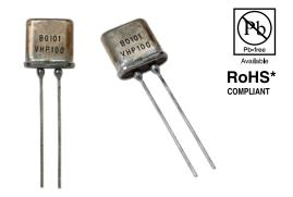
The VHP10x represents an essentially Zero Temperature Coefficient Resistor type of resistor. This oil filled hermetically sealed device makes unique use of foil on ceramic in such a way that self cancelling responses to temperature are produced by combining equal and opposite effects. This product is sold only in hermetic packages because applications requiring this level of temperature stability require humidity stability as well.
