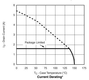
$^{\star}$  The power dissipation  $P_D$  is based on  $T_{J(max)}=150~^{\circ}C$ , using junction-to-case thermal resistance, and is more useful in settling the upper dissipation limit for cases where additional heatsinking is used. It is used to determine the current rating, when this rating falls below the package limit.
