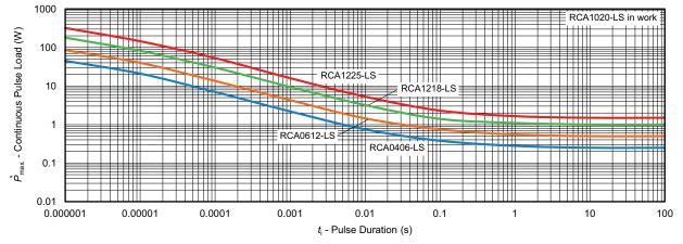
Maximum pulse load, continuous pulses; applicable if  $\bar{P} \leq P\left(\vartheta_{\rm amb}\right)$  and  $\hat{U} \leq \hat{U}_{\rm max}$ ; for permissible resistance change equivalent to 8000 h operation
