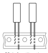
Case  $\emptyset$  D x L = 5 mm x 11 mm only Pitch F = 2.5 mm
