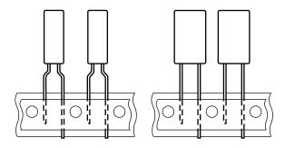
Case  $\emptyset$  D x L = 5 mm x 11 mm and 8.2 mm x 11 mm Pitch F = 5 mm
