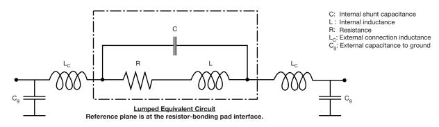
The lumped circuit above was used to model the data at the bonding pad-resistor reference plane. High frequency testing was performed by Modelithics, Inc. on parts mounted to quartz test boards. Quartz test boards were chosen to minimize the contribution of the board effects at high frequencies.
