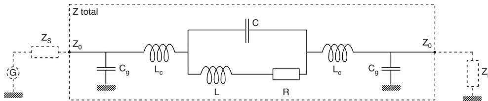
S-parameters are computed taking into account all the resistive, inductive and capacitive elements ( $Z_{total}$ ) and  $Z_0 = Z_L = Z_s = R$ .
