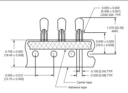
**Tape and Reel Specifications:** type 299D radial-leaded tantalum capacitors are available taped and reeled per EIA-468.
