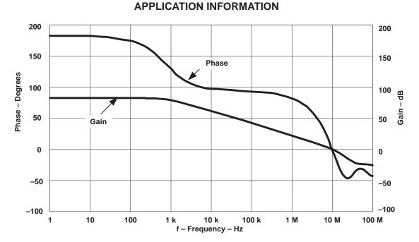
Figure 1. Error Amplifier Gain Phase Response
