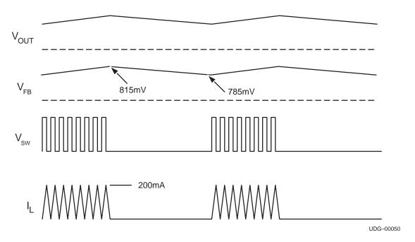
Figure 4. Typical Pulsed-Variable-Frequency Mode (PFM) Circuit Waveform
