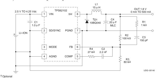
Figure 14. 1.8-V Output Automatic-Mode Switching Converter Application Circuit
