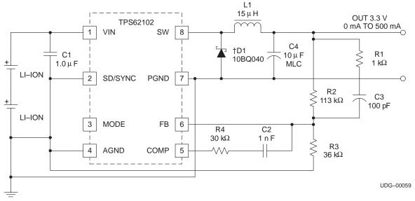
Figure 9. Automatic-Mode Switching Converter Application Circuit
