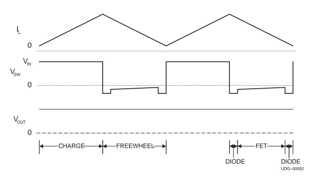
Figure 5. Typical Constant-Frequency Mode Circuit Waveforms
