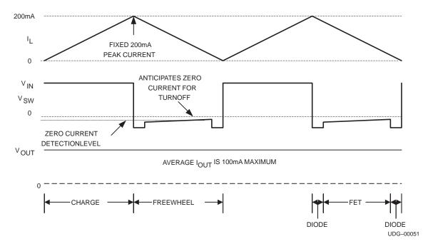
Figure 6. PFM Circuit Waveforms (Expanded View)
