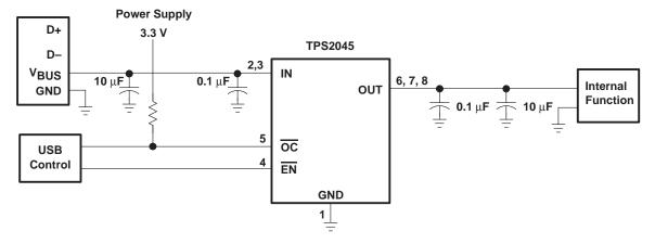
Figure 31. High-Power Bus-Powered Function
