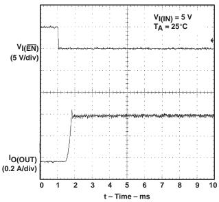
Figure 6. TPS2045, Short-Circuit Current,
