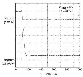
Figure 11. 1-Ω Load Connected to Enabled Device
