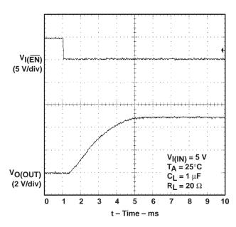
V<sub>I(EN)</sub> (5 V/div)  $V_{I(IN)} = 5 V$  $T_A = 25^{\circ}C$ VO(OUT)  $C_L = 1 \mu F$ (2 V/div)  $R_L = 20 \Omega$ 2 4 6 8 10 12 14 16 18 20 t - Time - ms
