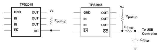
Figure 30. Typical Circuit for  $\overline{OC}$  Pin and RC Filter for Damping Inrush  $\overline{OC}$  Responses
