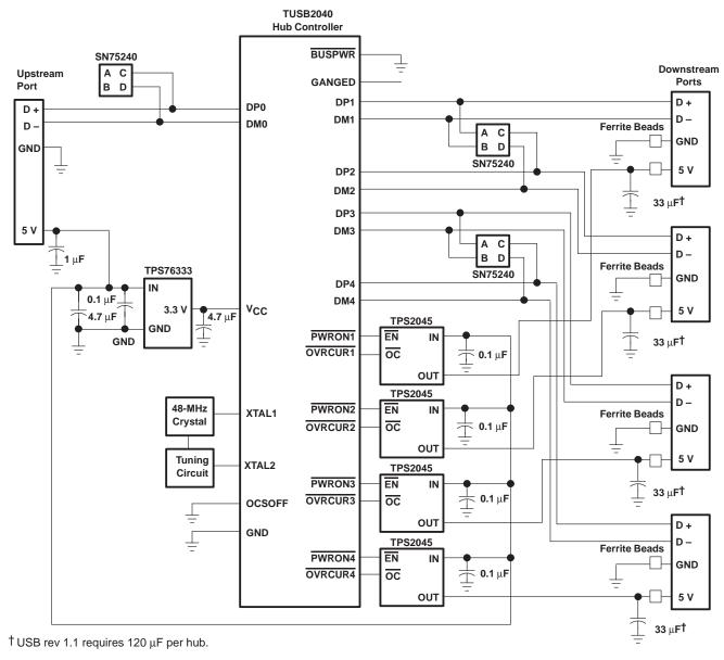
Figure 32. Bus-Powered Hub Implementation
