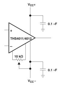
Figure 28. Offset Nulling Schematic
