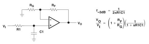
Figure 31. Single-Pole Low-Pass Filter
