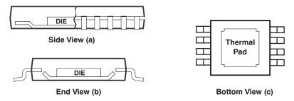
NOTE: The thermal pad is electrically isolated from all terminals in the package.
