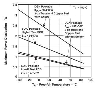
A. Results are with no airflow and PCB size =  $3 \text{ in } \times 3 \text{ in}$
