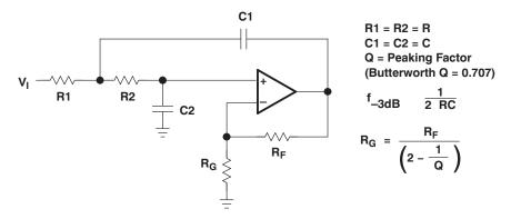
Figure 32. 2-Pole Low-Pass Sallen-Key Filter
