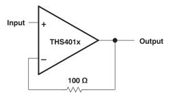
Figure 30. Noninverting Unity Gain Schematic
