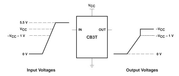
NOTE A: If the input high voltage (V<sub>IH</sub>) level is greater than or equal to V<sub>CC</sub> – 1 V, and less than or equal to 5.5 V, then the output high voltage (V<sub>OH</sub>) level will be equal to approximately the V<sub>CC</sub> voltage level.
