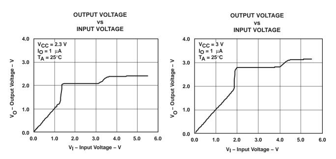
Figure 3. Data Output Voltage vs Data Input Voltage
