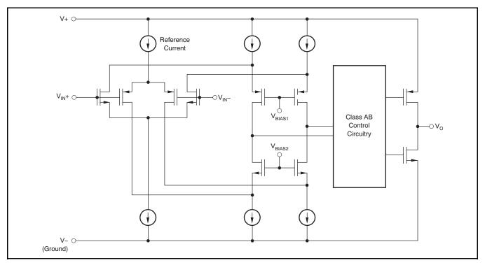
Figure 24. Simplified Schematic
