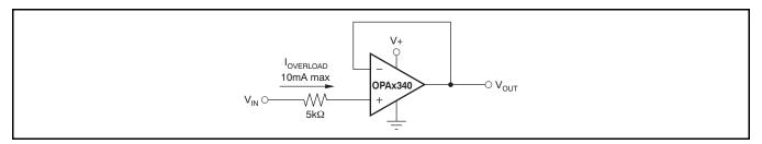
Figure 25. Input Current Protection for Voltages Exceeding the Supply Voltage
