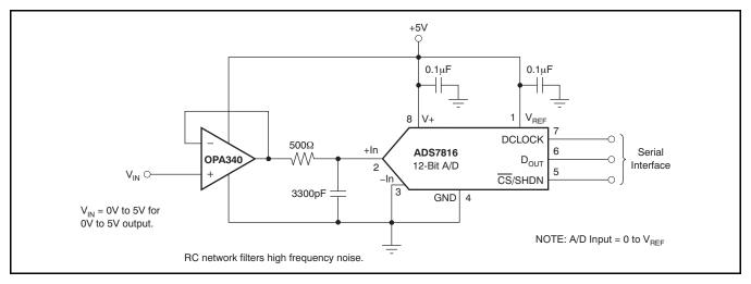
Figure 27. OPA340 in Noninverting Configuration Driving ADS7816
