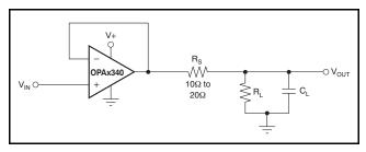
Figure 26. Series Resistor in Unity-Gain Configuration Improves Capacitive Load Drive
