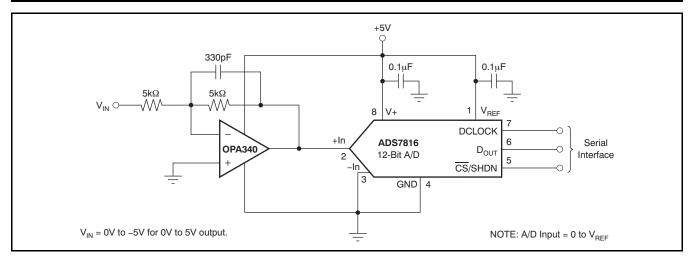
Figure 28. OPA340 in Inverting Configuration Driving ADS7816
