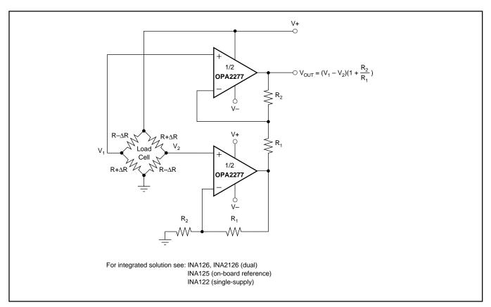
FIGURE 3. Load Cell Amplifier.
