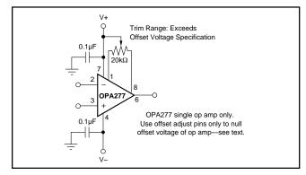
FIGURE 1. OPA277 Offset Voltage Trim Circuit.
