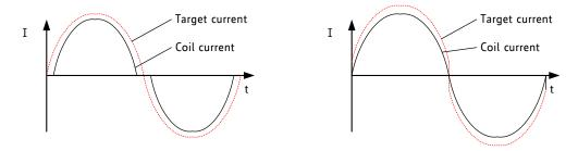
Figure 8.5 Zero crossing with classic chopper and correction using sine wave offset
