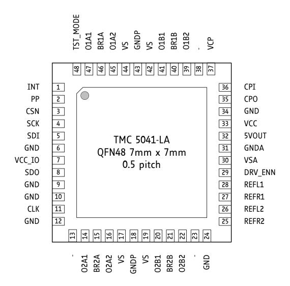
Figure 2.1 TMC5041 pin assignments.
