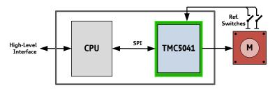
Two reference switch inputs can be used for each motor. A single CPU controls the whole system, which is highly economical and space saving, because the TMC5041 covers all functionality required to drive the motor.
