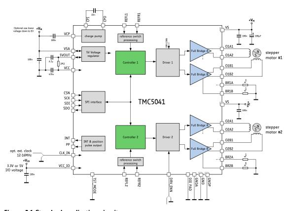
Figure 3.1 Standard application circuit
