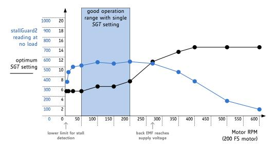
Figure 11.2 Example: Optimum SGT setting and stallGuard2 reading with an example motor
