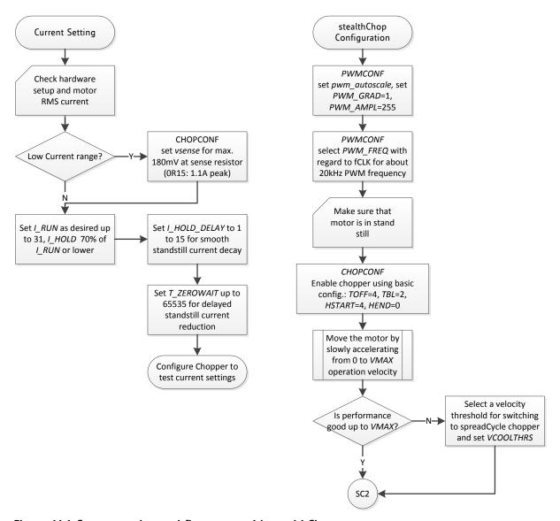
Figure 14.1 Current setting and first steps with stealthChop
