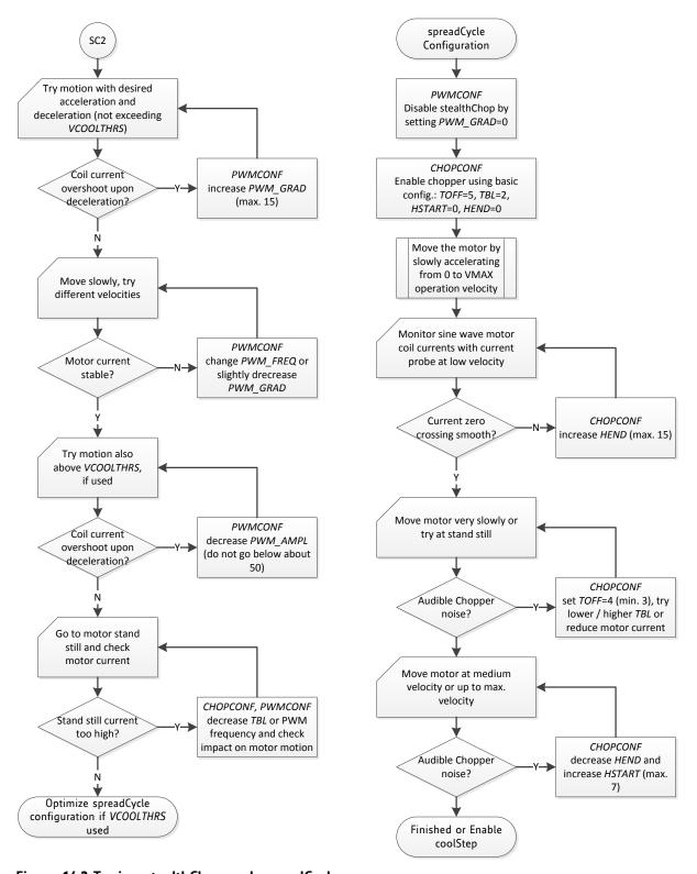
Figure 14.2 Tuning stealthChop and spreadCycle
