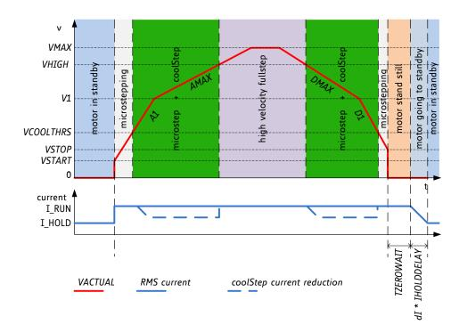
Figure 10.3 Ramp generator velocity dependent motor control
