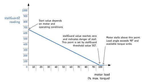
Figure 11.1 Function principle of stallGuard2
