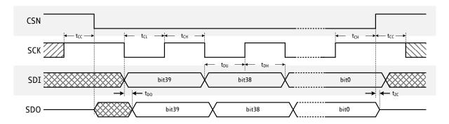
Figure 4.1 SPI timing
