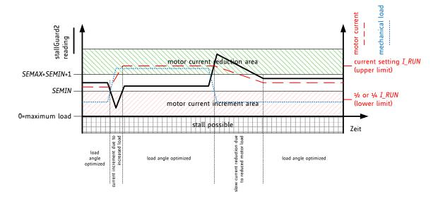
Figure 12.1 coolStep adapts motor current to the load
