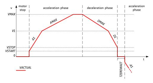
Figure 10.1 Ramp generator velocity trace showing consequent move in negative direction
