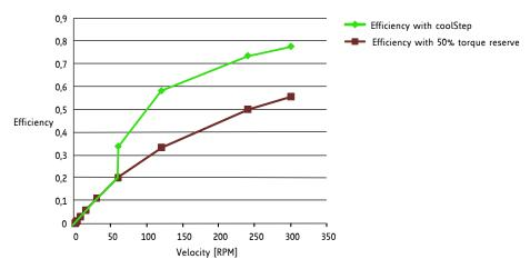
Figure 1.2 Energy efficiency with coolStep (example)
