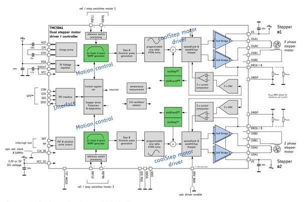
Figure 1.1 Basic application and block diagram
