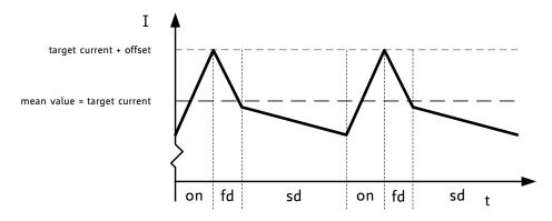
Figure 8.4 Classic const. off time chopper with offset showing coil current
