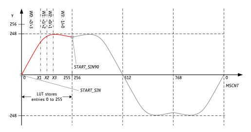
Figure 13.1 LUT programming example
