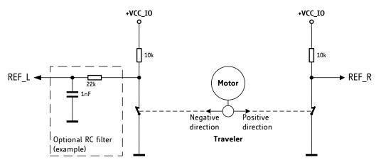
Figure 10.4 Using reference switches (example)
