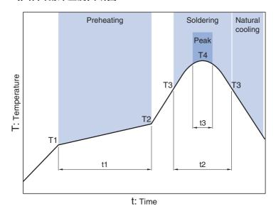
Preheating Soldering Peak Temp. Time Temp. Time Temp. Time T2 **T4** T1 t2 t1 Т3 t3 150°C 180°C 60 to 120s 230°C 30s 260°C 10s
