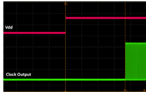
Figure 16. Startup Waveform vs. Vdd
