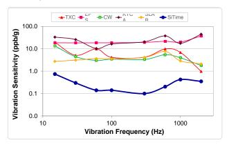
Figure 5. Vibration Robustness<sup>[5]</sup>
