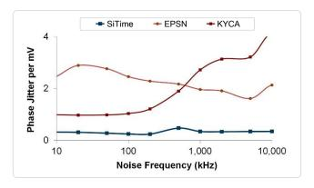
Figure 4. Power Supply Noise Rejection<sup>[4]</sup>
