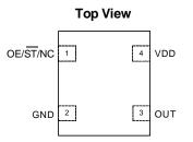
Figure 1. Pin Assignments
