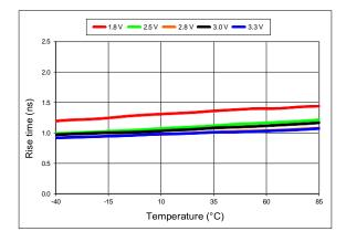
Figure 12. 20%-80% Rise Time vs Temperature
