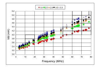
Figure 8. Idd vs Frequency
