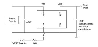
Figure 2. Test Circuit
