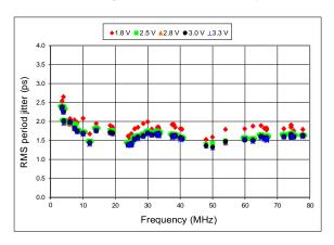
Figure 10. RMS Period Jitter vs Frequency
