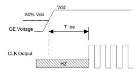
T\_oe: Time to re-enable the clock output
