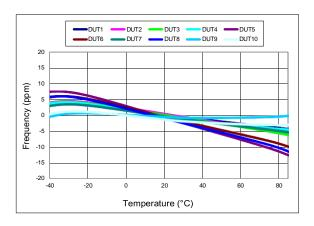
Figure 9. Frequency vsTemperature
