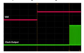
Figure 17. Startup Waveform vs. Vdd
