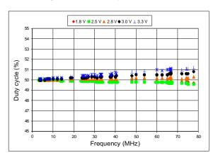
Figure 11. Duty Cycle vs Frequency
