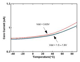
Figure 8. Core Current Over Temperature
