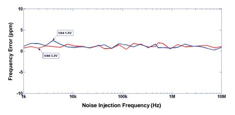
Figure 11. Power Supply Noise Rejection (±150mV Noise)
