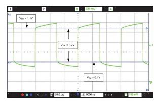
Figure 4. SiT1532AI-J4-<u>D14</u>-32.768 Output Waveform (10 pF load)
