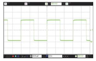
Figure 13. LVCMOS Output Waveform ( $V_{swing} = 1.8V$ , SiT1532AI-J4-DCC-32.768)
