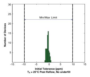
Figure 6. Initial Tolerance Histogram
