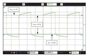
Figure 12. NanoDrive<sup>TM</sup> Output Waveform ( $V_{OH} = 1.1V$ ,  $V_{OL} = 0.4V$ ; SiT1532AI-J4-D14-32.768)
