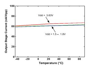
Figure 9. Output Stage Current Over Temperature
