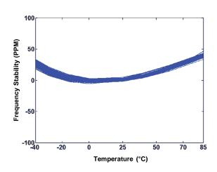
Figure 7. Frequency Stability Over Temperature
