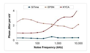
Figure 4. Power Supply Noise Rejection[4]
