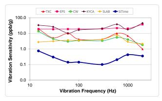
Figure 5. Vibration Robustness<sup>[5]</sup>
