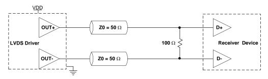
Figure 6. LVDS Single Termination (Load Terminated)
