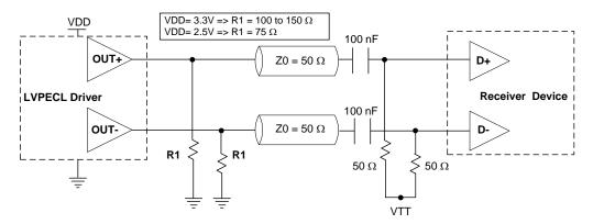
Figure 4. LVPECL AC Coupled Termination
