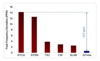
Figure 6. Shock Robustness<sup>[6]</sup>
