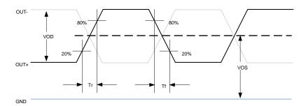
Figure 2. LVDS Voltage Levels per Differential Pin (OUT+/OUT-)
