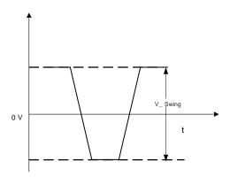
Figure 1(b). LVPECL Voltage Levels Across Differential Pair
