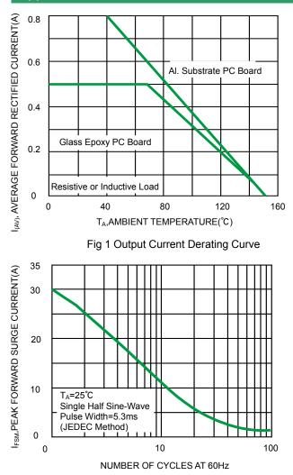
Fig 3.Maximum Peak Forward Surge Current(per leg)
