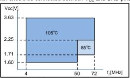
Please note that Supply voltage range (V<sub>CC</sub>) depends on Output frequency(fo) and upper limit of Operating temperature(T\_use Max.).
