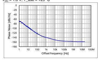
Phase Jitter (Offset frequency: 12 kHz to 20 MHz)
