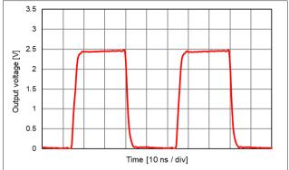
$V_{CC} = 1.8 \text{ V}, L\_CMOS = 15 \text{ pF}, T\_use = +25 ^{\circ}C$
