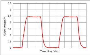
$V_{CC} = 1.8 \text{ V}, L\_CMOS = 15 \text{ pF}, T\_use = +25 ^{\circ}C$
