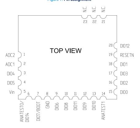
Figure 7. Pin assignment
