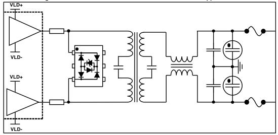
On topologies given in Figure 8: "xDSL and G.FAST schematic for CPE applications" and Figure 9: "xDSL and G.FAST schematic for infrastructure applications", +VLD and -VLD may not be connected.
