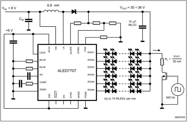
Figure 19. Load transient response measurement setup
