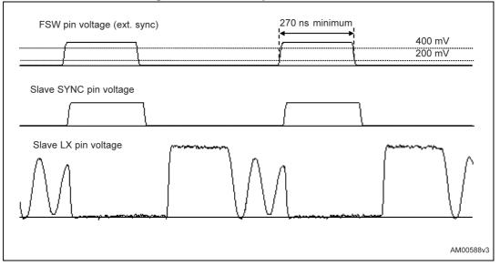
Figure 11. External sync. waveforms
