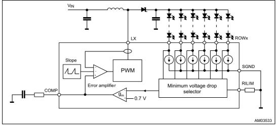
Figure 5. Main loop and current loop diagram
