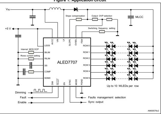
Figure 1. Application circuit
