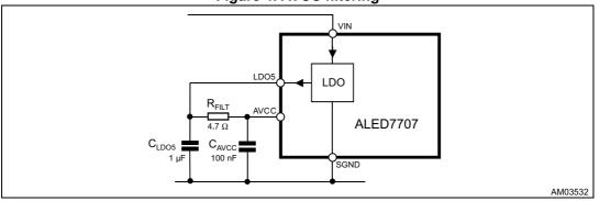
Figure 4. AVCC filtering
