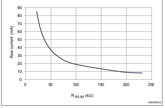
Figure 13. Row current vs R<sub>RILIM</sub>
