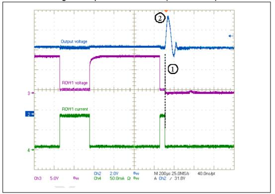
Figure 16. Open channel detection (MODE to AVCC)
