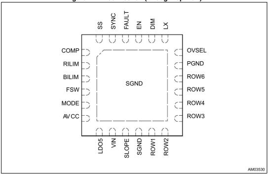
Figure 2. Pin connection (through top view)
