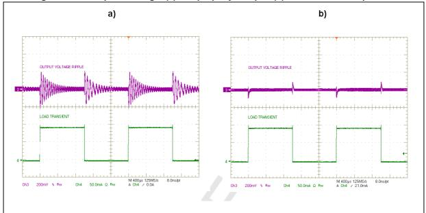
Figure 18. Poor phase margin (a) and properly damped (b) load transient responses
