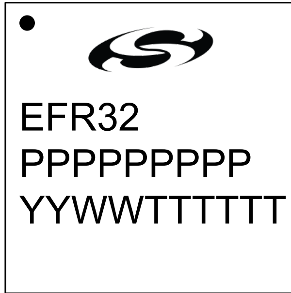
Figure 8.3. QFN32 Package Marking
