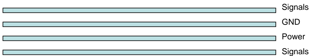
Figure 15: Typical 4-layer PCB construction
