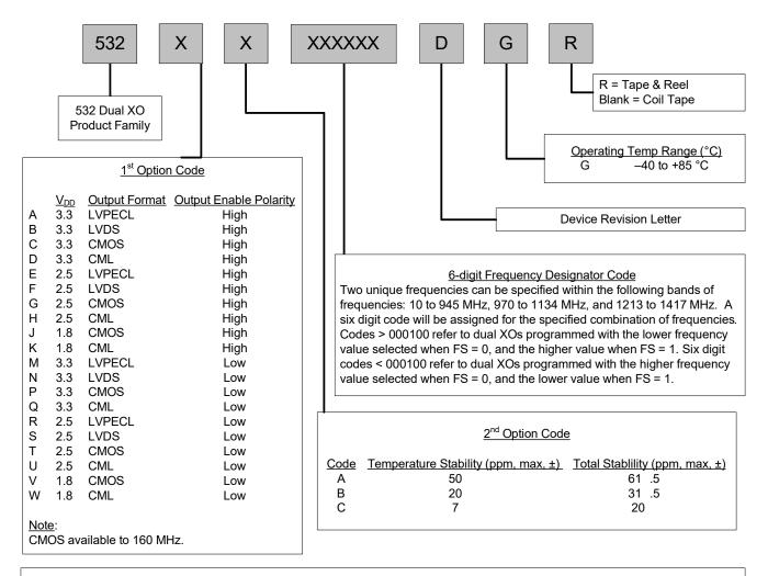
Example Part Number: 532AB000108DGR is a  $5 \times 7$  mm Dual XO in a 6 pad package. Since the six digit code (000108) is > 000100, f0 is 644.53125 MHz (lower frequency) and f1 is 693.48299 (higher frequency), with a 3.3 V supply, LVPECL output, and Output Enable active high polarity. Temperature stability is specified as  $\pm 20$  ppm. The part is specified for a -40 to  $\pm 85$  C° ambient temperature range operation and is shipped in tape and reel format.
