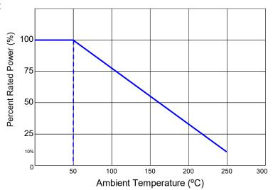
Note: This curve assumes the part is mounted on a properly sized heat sink.
