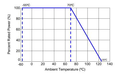
High Value Thick Film Chip Resistor
