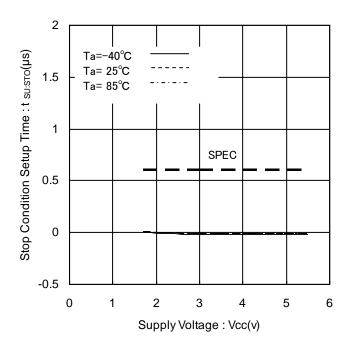
Figure 24. Stop Condition Setup Time vs Supply Voltage
