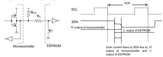
Figure 45. I/O Circuit Diagram
