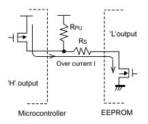
Figure 48. I/O Circuit Diagram
