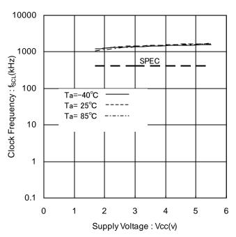
Figure 13. Clock Frequency vs Supply Voltage
