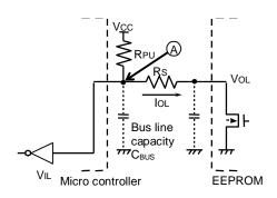
Figure 47. I/O Circuit Diagram
