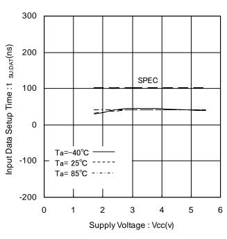
Figure 21. Input Data Setup Time vs Supply Voltage (LOW)
