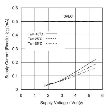
Figure 11. Supply Current (Read) vs Supply Voltage (fsct=400kHz)
