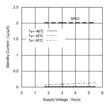
Figure 12. Standby Current vs Supply Voltage
