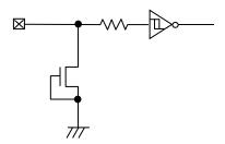
Figure 49. Input Pin Circuit Diagram
