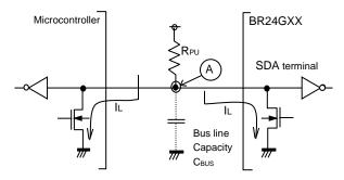
Figure 44. I/O Circuit Diagram
