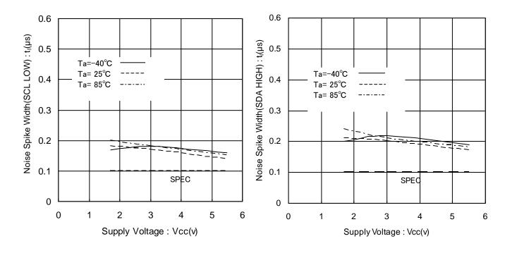
Figure 28. Noise Spike Width vs Supply Voltage (SCL LOW)
