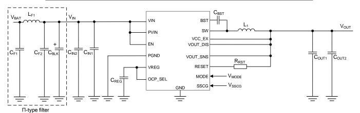
Figure 62. Reference Circuit 2
