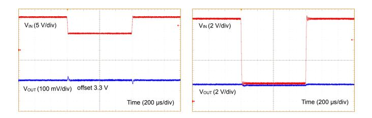
Figure 69. Line Response 1  $(V_{IN} = 16 \text{ V to } 8 \text{ V}, I_{OUT} = 1 \text{ A})$
