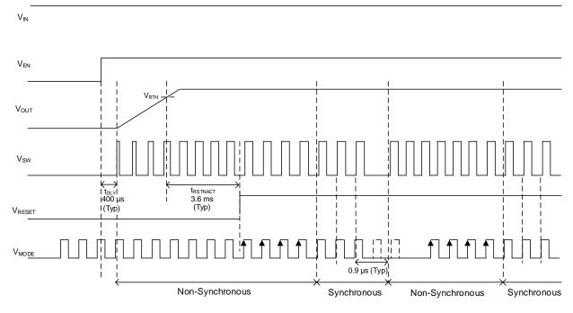
Figure 35. External Synchronization Function
