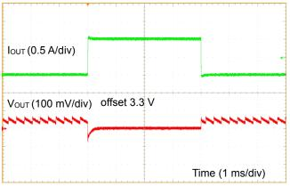
Figure 67. Load Response 1 (V<sub>IN</sub> = 12 V, V<sub>MODE</sub> = 5 V, I<sub>OUT</sub> = 0 A to 1 A)
