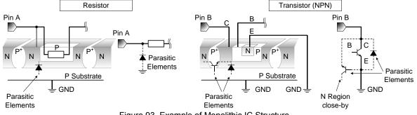
Figure 93. Example of Monolithic IC Structure
