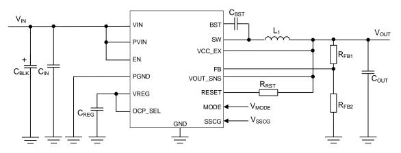
Figure 47. Application Sample Circuit
