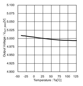
Figure 12. Output Voltage vs Temperature (BD9P155MUF-C)
