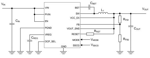
Figure 3. Application Circuit (BD9P105MUF-C)
