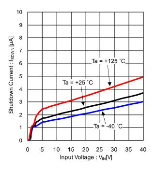
Figure 9. Shutdown Current vs Input Voltage
