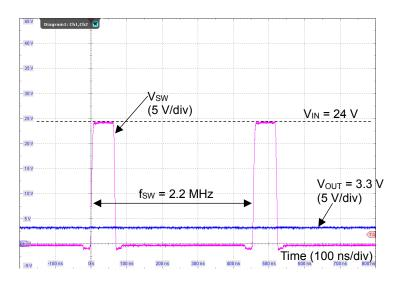
Figure 29. Switching Waveform (V<sub>IN</sub> = 24 V, V<sub>OUT</sub> = 3.3 V, I<sub>OUT</sub> = 0.5 A,  $f_{SW}$  = 2.2 MHz)
