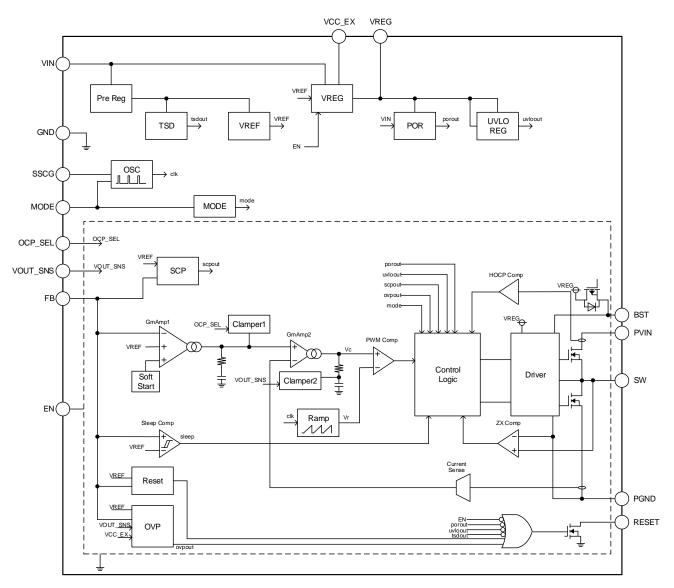
Figure 7. Block Diagram (BD9P105MUF-C)
