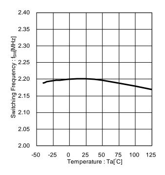
Figure 19. Switching Frequency vs Temperature
