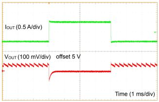
Figure 80. Load Response 1 ( $V_{IN}$  = 12 V,  $V_{MODE}$  = 5 V,  $I_{OUT}$  = 0 A to 1 A)
