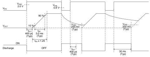
Figure 33. Enable ON/OFF Timing Chart
