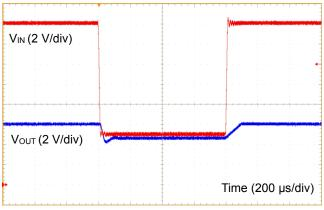
Figure 56. Line Response 1  $(V_{IN} = 16 \text{ V to } 8 \text{ V}, I_{OUT} = 1 \text{ A})$
