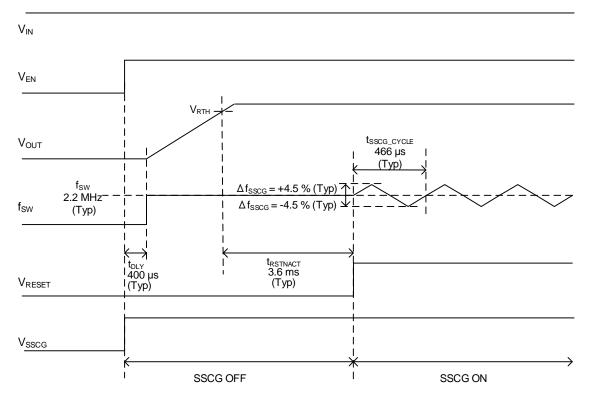
Figure 37. Spread Spectrum Function
