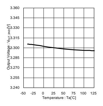
Figure 11. Output Voltage vs Temperature (BD9P135MUF-C)
