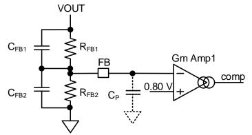
Figure 48. Setting for Output Setting Resistor
