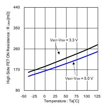
Figure 21. High Side FET ON Resistance vs Temperature
