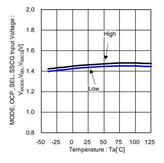
Figure 17. MODE, OCP\_SEL, SSCG Input Voltage vs Temperature
