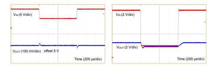
Figure 82. Line Response 1 ( $V_{IN}$  = 16 V to 8 V,  $I_{OUT}$  = 1 A)
