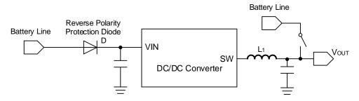
Figure 46. VOUT shorted to Battery Line
