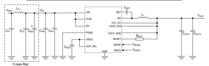
Figure 75. Reference Circuit 3
