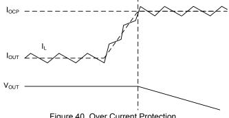
Figure 40. Over Current Protection
