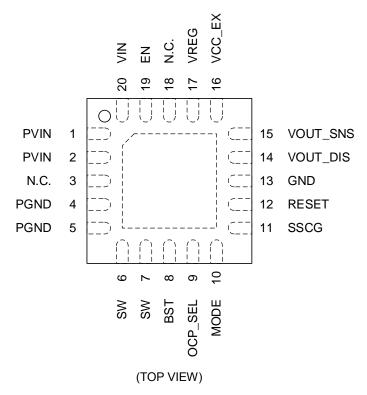
Figure 5. Pin Configuration (BD9P135MUF-C, BD9P155MUF-C)
