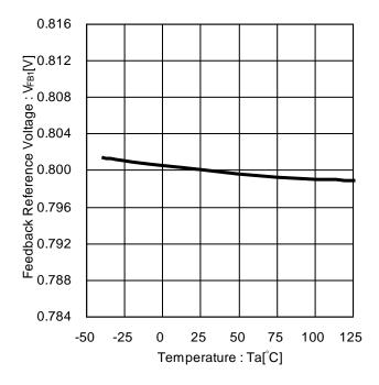
Figure 10. Feedback Reference Voltage vs Temperature (BD9P105MUF-C)
