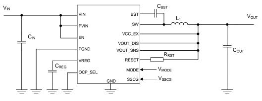
Figure 1. Application Circuit with Discharge Function (BD9P135MUF-C, BD9P155MUF-C)
