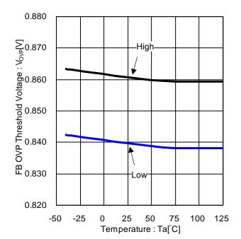
Figure 26. FB OVP Threshold Voltage vs Temperature (BD9P105MUF-C)
