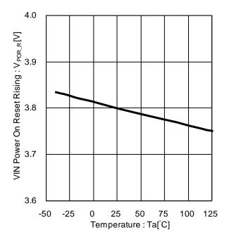
Figure 13. VIN Power On Reset Rising vs Temperature
