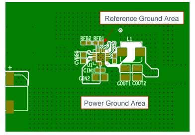
Figure 90. Recommended Board Layout Example (for BD9P1x5MUF-C)
