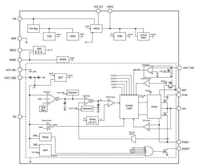
Figure 8. Block Diagram (BD9P135MUF-C, BD9P155MUF-C)
