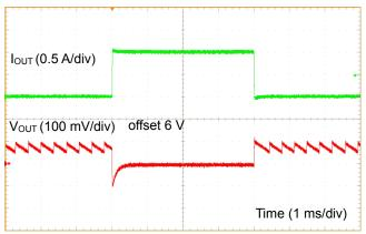
Figure 54. Load Response 1 (V\_{IN} = 12 V, V\_{MODE} = 5 V, I\_{OUT} = 0 A to 1 A)
