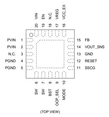
Figure 6. Pin Configuration (BD9P105MUF-C)
