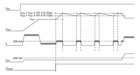
Figure 32. Timing Chart in Light Load Mode after Detecting RESET High (OCP\_SEL = H)
