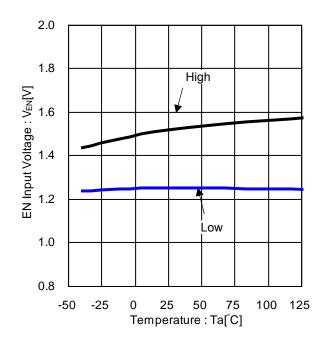
Figure 15. EN Input Voltage vs Temperature
