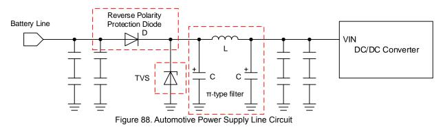
As a reference, the automotive power supply line circuit example is given in figure above.
