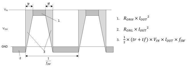
Figure 92. SW Waveform
