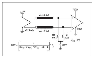
Figure 5A. 3.3V LVPECL Output Termination
