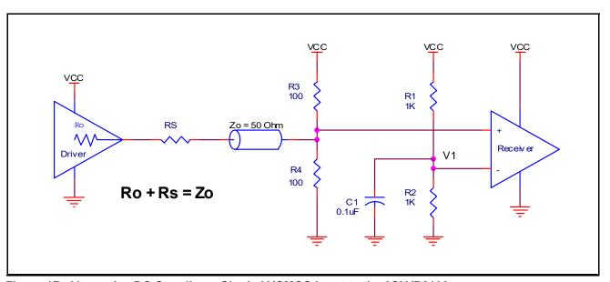
Figure 1B. Alternative DC Coupling a Single LVCMOS Input to the 8SLVP2108
