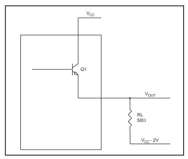
Figure 7. LVPECL Driver Circuit and Termination
