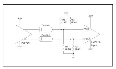
Figure 3A. PCLK/nPCLK Input Driven by a 2.5V LVPECL Driver
