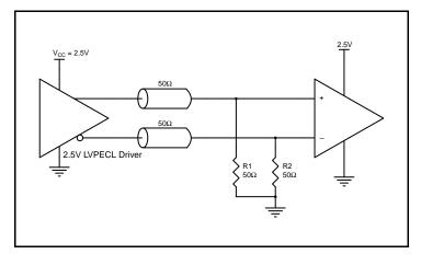
Figure 6C. 2.5V LVPECL Driver Termination Example
