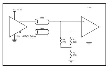
Figure 6B. 2.5V LVPECL Driver Termination Example
