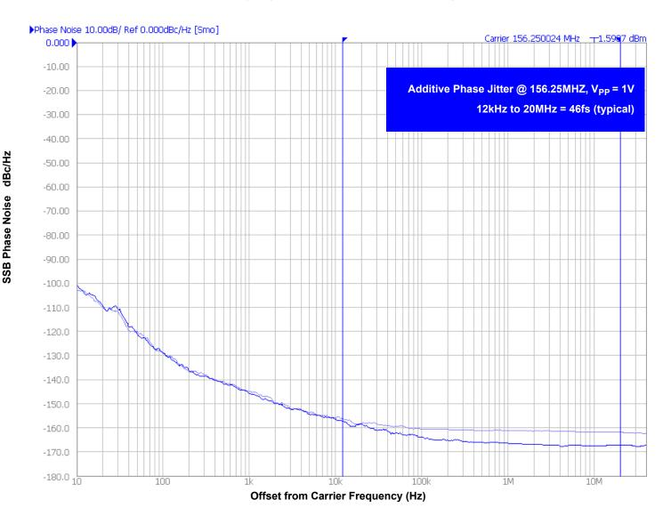
As with most timing specifications, phase noise measurements have issues relating to the limitations of the equipment. Often the noise floor of the equipment is higher than the noise floor of the device. This is illustrated above. The device meets the noise floor of what is
