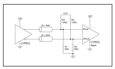
Figure 2A. PCLK/nPCLK Input Driven by a 3.3V LVPECL Driver
