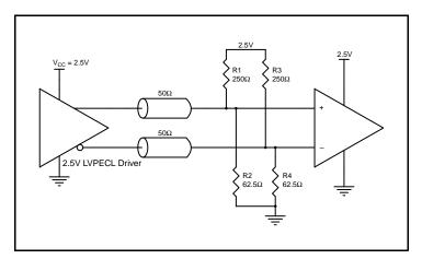
Figure 6A. 2.5V LVPECL Driver Termination Example
