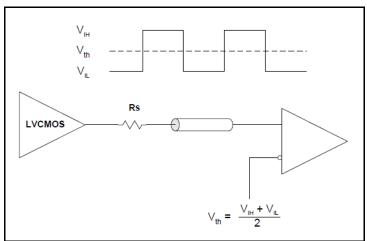
Figure 1A. DC-Coupling a Single LVCMOS Input to the 8SLVP2108
