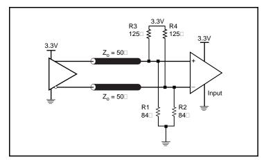
Figure 5B. 3.3V LVPECL Output Termination
