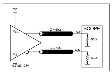
2.5V LVPECL Output Load Test Circuit
