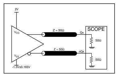
3.3V LVPECL Output Load Test Circuit
