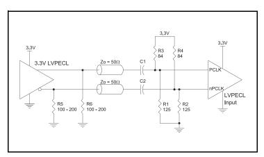
Figure 2B. PCLK/nPCLK Input Driven by a 3.3V LVPECL Driver with AC Couple
