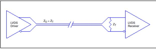
Figure2A. Standard LVDS Termination
