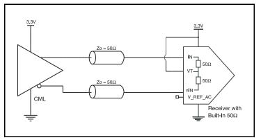
Figure1B. IN/nIN Input with Built-In 50 $\Omega$ Driven by a CML Driver with Open Collector
