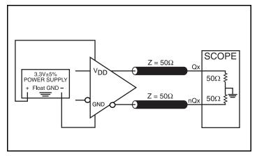
LVDS Output Load AC Test Circuit
