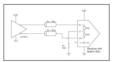
Figure1C. IN/nIN Input with Built-In 50  $\Omega$  Driven by an LVPECL Driver
