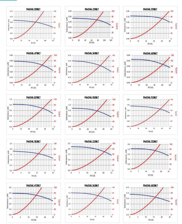
High Current Molded Power Inductor - PA4346 & PM4346 Series
