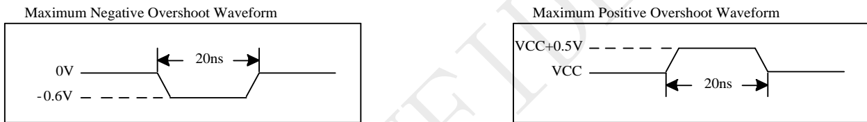
Figure 5-1 Maximum Overshoot Waveform
