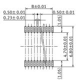
Recommended metal mask pattern Metal mask thickness: When 120 µm (Opening area ratio: 72%)
