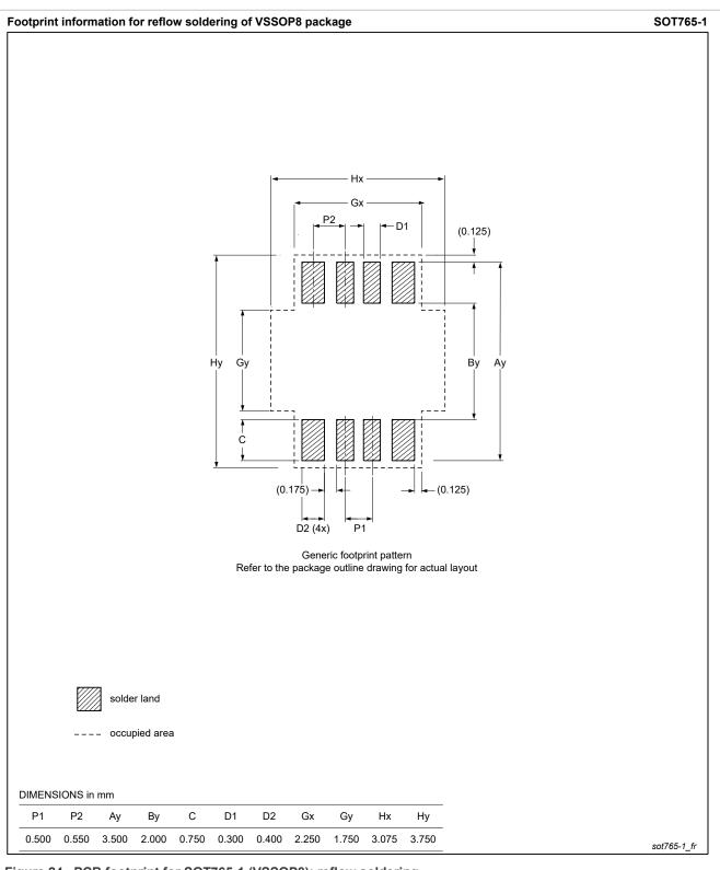
Figure 24. PCB footprint for SOT765-1 (VSSOP8); reflow soldering
