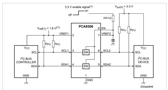
1. In the Enabled mode, the applied enable voltage and the applied voltage at  $V_{ref(1)}$  should be such that  $V_{bias(ref)(2)}$  is at least 1 V higher than  $V_{ref(1)}$  for best translator operation.
