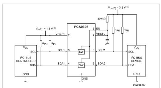
1. The applied voltages at  $V_{ref(1)}$  and  $V_{pu(D)}$  should be such that  $V_{bias(ref)(2)}$  is at least 1 V higher than  $V_{ref(1)}$  for best translator operation.
