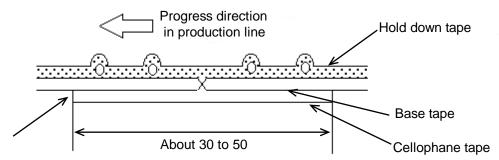
No lifting for the direction of progressing
