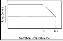
■ Operating Temperature : -55°C to +125°C ■ Storage Temperature : -55°C to +125°C
