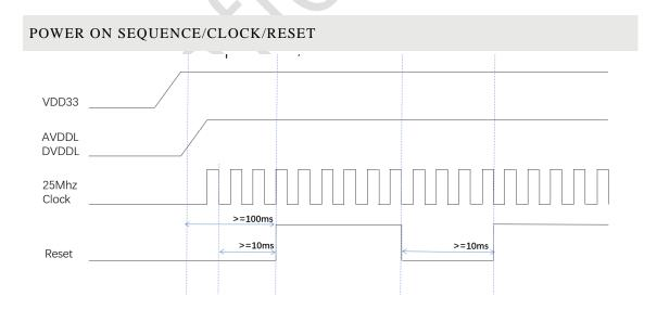
When using crystal, the clock is generated internally after power is stable. For a reliable power on reset, suggest to keep asserting the reset low long enough (100ms) to ensure the clock is stable and clock-to-reset 10ms requirement is satisfied.
