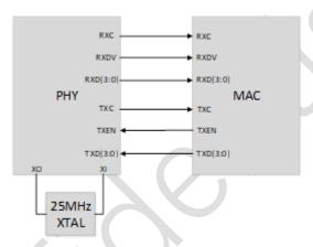
Figure . connection diagram of MII
