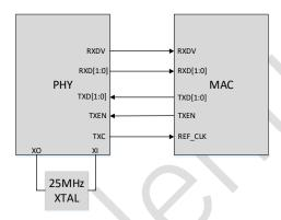
Figure .connection diagram of RMII2
