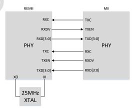
Figure .connection diagram of REMII
