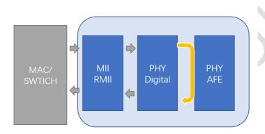
Figure . Internal loopback
